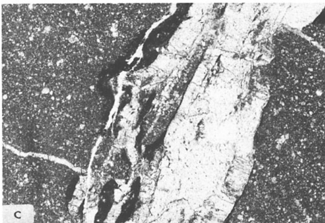
Figure 6c. Photomicrograph showing overprinting relationship between strike (thick) and bedding parallel (thin) veins (plane polarized light; field of view, 2.5×2.8 mm).
