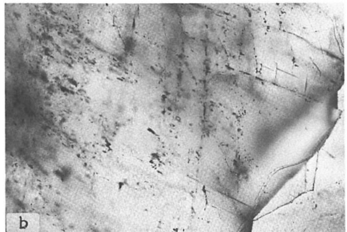
Figure 8b. Photomicrograph showing two-phase (L-V), primary fluid inclusions along the growth zones in calcite from bedding-parallel veins (plane polarized light; field of view, 0.3×0.5 mm).
