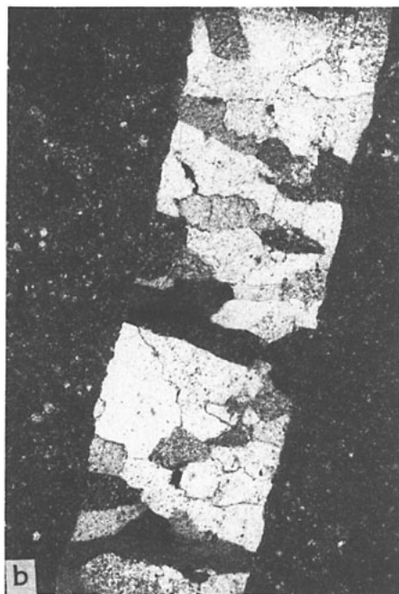
Figure 7b. Photomicrograph showing sharp and rectilinear boundaries of cross-fold vein. The crystallographic continuity of fibers from wall to wall is noteworthy (crossed nicols; field of view, 2.5x2.8 mm).
