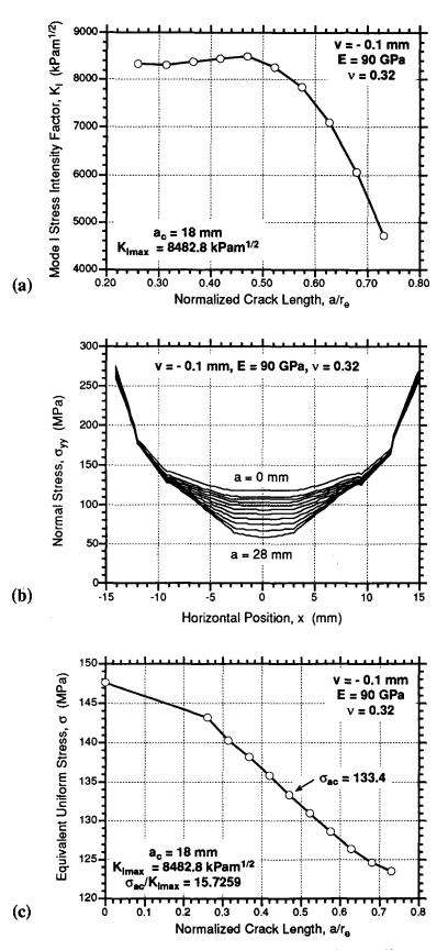
Fig. 10. Variation in  $K_1$  (a), horizontal distribution of normal stress,  $\sigma_{yy}$ , (b) and equivalent uniform stress,  $\sigma$  (c) during crack growth in a MRS specimen compressed by 0.1 mm, and with material properties of E = 90 GPa, and  $\nu = 0.32$  under slip-allowed conditions. Except for the order of magnitude difference in E, all aspects of this model are identical to the model used to calculate the results in Fig. 9.
