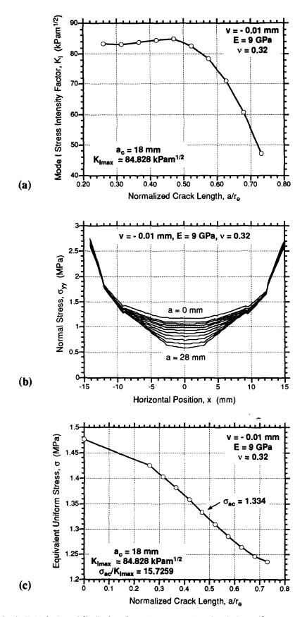
Fig. 11. Variation in  $K_1$  (a), horizontal distribution of normal stress,  $\sigma_{yy}$ , (b) and equivalent uniform stress,  $\sigma$  (c) during crack growth in a MRS specimen compressed by 0.01 mm, and with material properties of E = 9 GPa, and v = 0.32 under slip-allowed conditions. Except for the order of magnitude difference in v, all aspects of this model are identical to the model used to calculate the results in Fig. 9.
