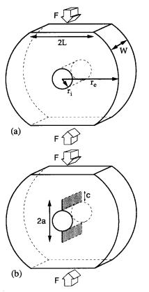
Fig. 1. Geometry of modified ring test specimens: (a) initial modified ring specimen; (b) crack geometry in a modified ring specimen.
