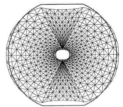
Fig. 13. Geometry of deformation in an MRS specimen when constant stress of 2.238 MPa is applied directly to the specimen loading surfaces, and slip is allowed between the specimen and loading platen. Thick gray lines represent the original shape of the specimen. Deformation magnified 500 times for illustration. Similar deformation occurs when slip is not allowed at the specimen-platen interface.
