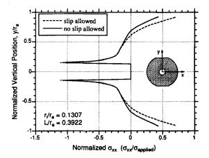
Fig. 7. Influence of specimen-platen interaction on the initial distribution of  $\sigma_{xx}$  along the y-axis of an MRS specimen subjected to constant forces along the loading surfaces.
