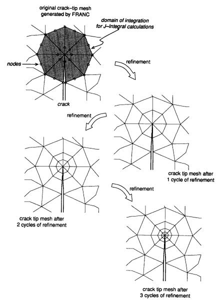
Fig. 5. Method of mesh refinement in FRANC. Note that the area utilized in calculating the *J*-integral is constant, but that the number of elements in the domain of integration increases by a factor of two during each successive refinement cycle.
