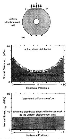
Fig. 8. Calculation of equivalent uniform stress: (a) location of measurement for  $\sigma_{yy}$  distribution; (b) schematic distribution of  $\sigma_{yy}$  observed along specimen loading surface; (c) schematic equivalent uniform stress with the same integrated stress as in (b).
