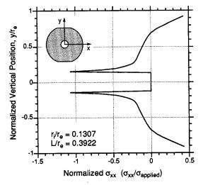
Fig. 2. Numerical solution for the distribution of  $\sigma_{xx}$  along the y-axis of a modified ring specimen under vertical compression.
